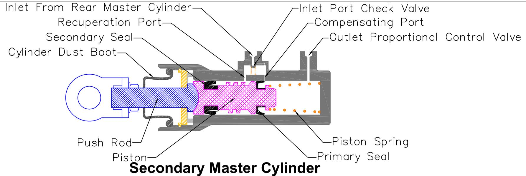
The Honda ST1300 uses (in addition to the front master-cylinder (lever), and the rear master-cylinder (pedal)) a third brake master-cylinder to operate the two non-center pistons of the rear brake caliper. The Secondary Master Cylinder (SMC) is applied only when the motorcycle is moving forward and either the front or rear master-cylinder is activated. Thus it is the SMC that is responsible for linking the front wheel brake with the rear wheel brake.
